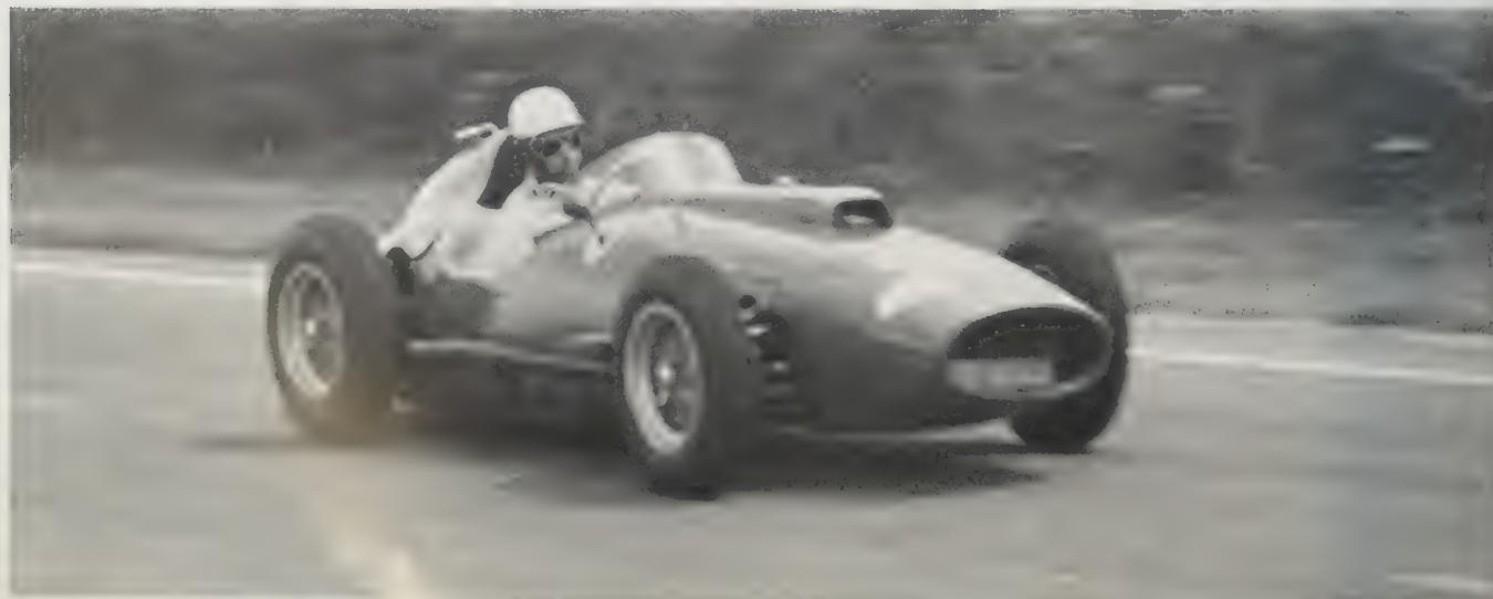
Right: Lampredi-designed 60 deg V-6 1490 cc Formula 2 car, seen here at Reims where Maurice Trintignant won the 1957 Coupe de Vitesse.
