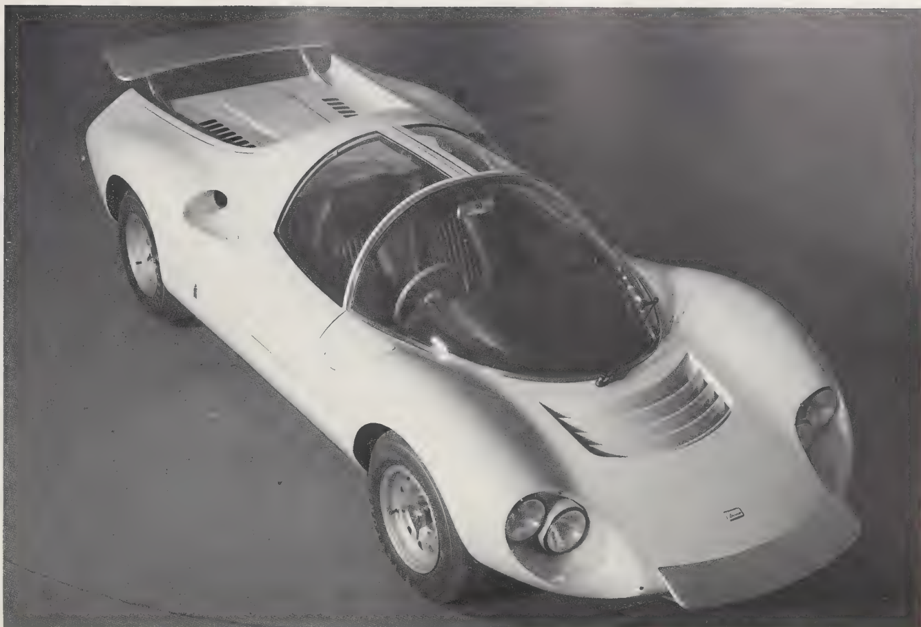
Opposite, right and below: 1967 prototype Dino 206GT with front/rear spoilers and gull-wing doors. This was more a research vehicle than a real racing body.
